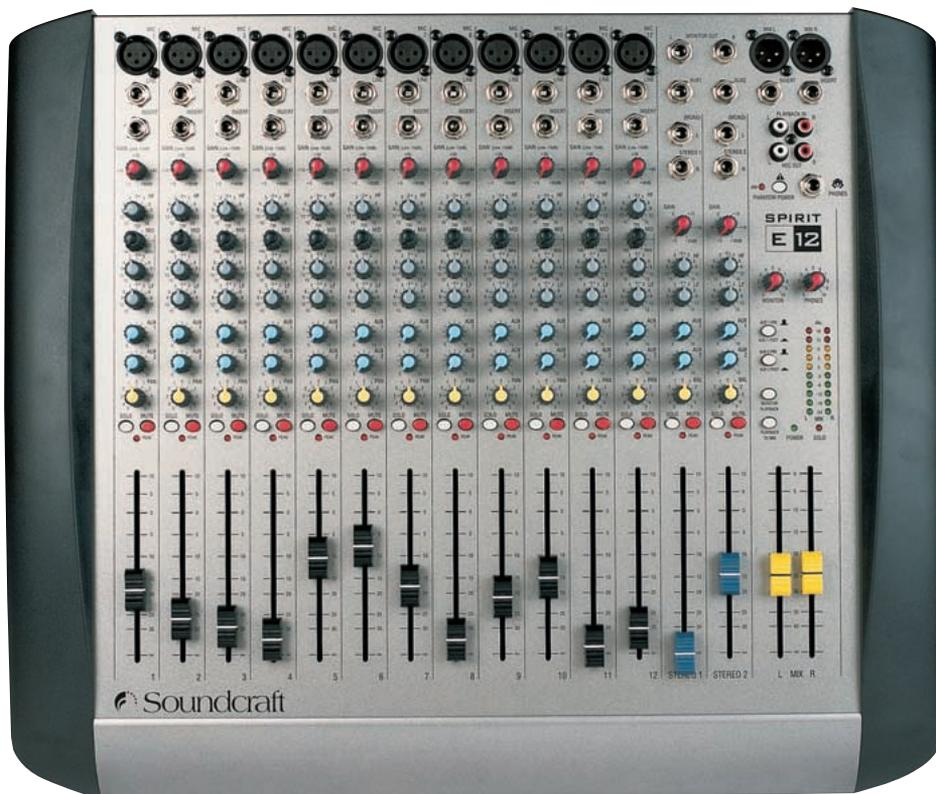
The colour coding of pots and faders makes the E12 simple to use
